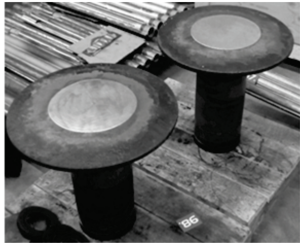
Fig. 1. Buffer heads covered with a layer of aluminium bronze.
