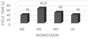
Fig. 5. Analysis of cycle times in individual FAL cells.
