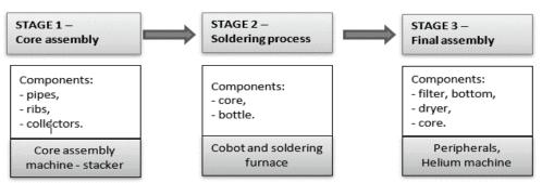
Fig. 2. Production stages of the condenser.
