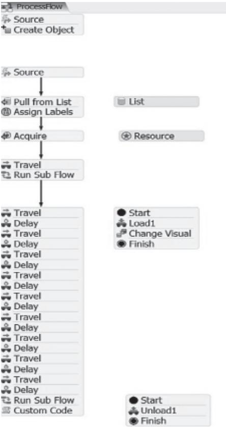
Fig. 6. Algorithm of rail transport using Process Flow module.
