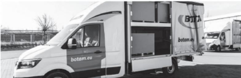
Fig. 3. Double floor in a vehicle with a GVM <3.5 t
